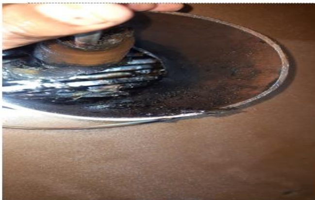
Damage at HV take-off point Y-Ph winding.
