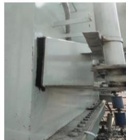
Ruptured Tank Stiffener
