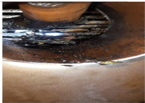
Damage at HV take-off point Y-Ph winding.
