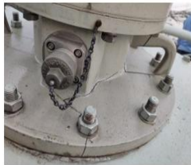
Crack observed on HV Bushings Flange
