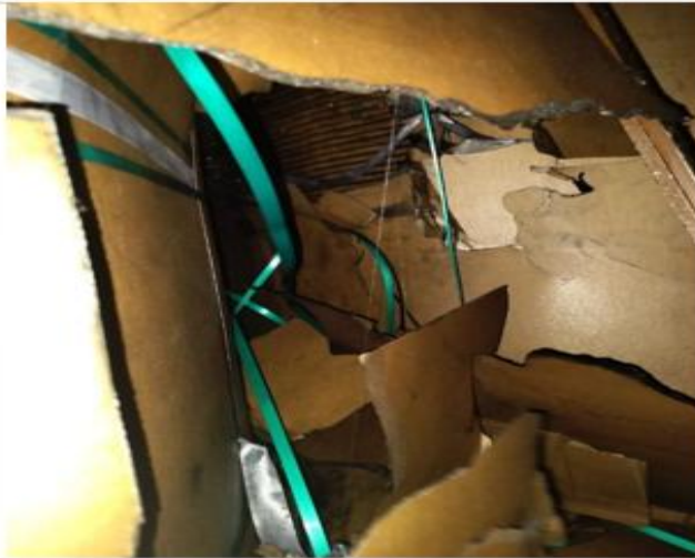
Broken pressboard & barriers of series winding of Y & B Phase
