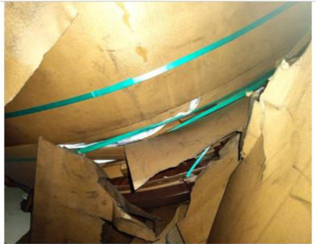
Broken pressboard & barriers of series winding of Y & B Phase
